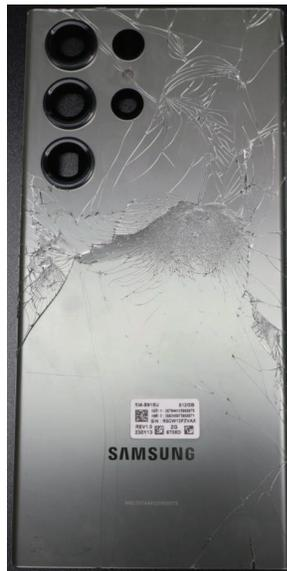
When repairing a device with a severely damaged backglass, be aware that components underneath, like the Main and/or Sub PBA and rear cameras, may also be affected and should be inspected thoroughly.
