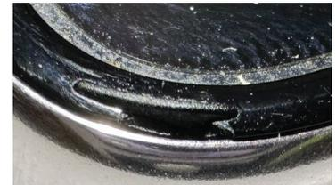
Any cracks, chips, gouges, or missing pieces of the deco should be considered OOW
