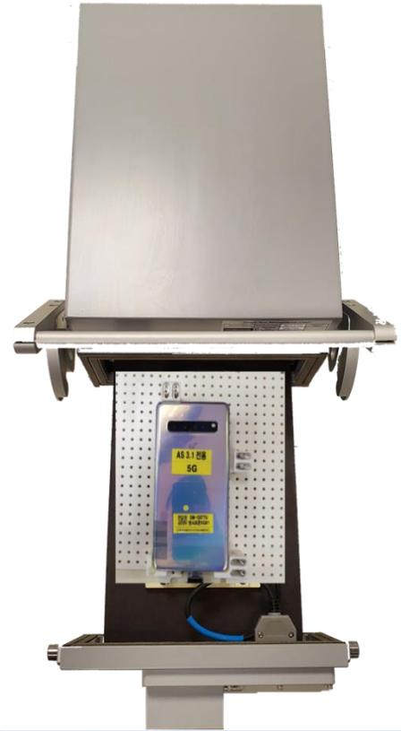
**Note:** Do not pull the chamber drawer all the way out; this will derail the chamber from its sliding tracks
