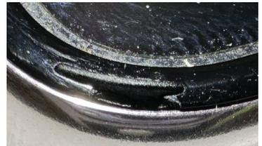
If the deco or p-cap has any chips, cracks, or missing pieces the repair is considered out of warranty and should be charged to the customer
