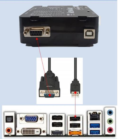
**Note:** Connecting the Anyway Jig to the Service PC will generate a COM Port for the Anyway Jig, which can be found in the Windows Device Manager
