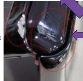
Excessive damage to the outside of the device, especially on or around the hinge can also directly void the warranty of the display on the other side.
